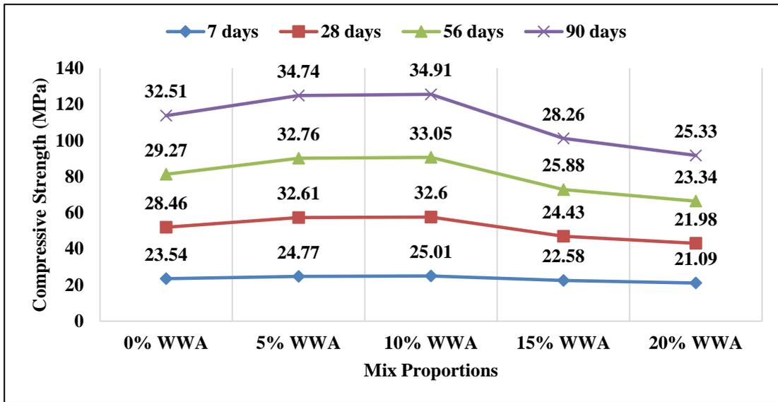
Figure 4- Compressive Strength of WWA Concrete
