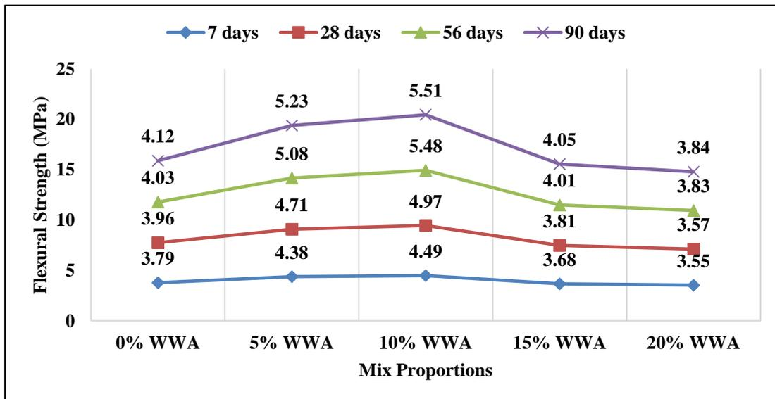
Figure 6- Flexural Strength of WWA Concrete
