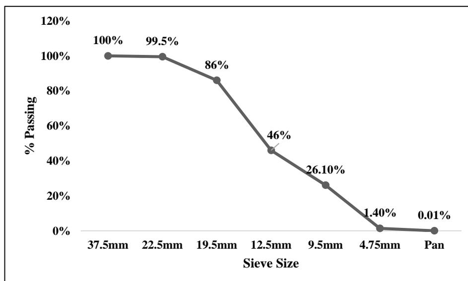
Figure 2- Gradation Curve of Coarse Aggregates
