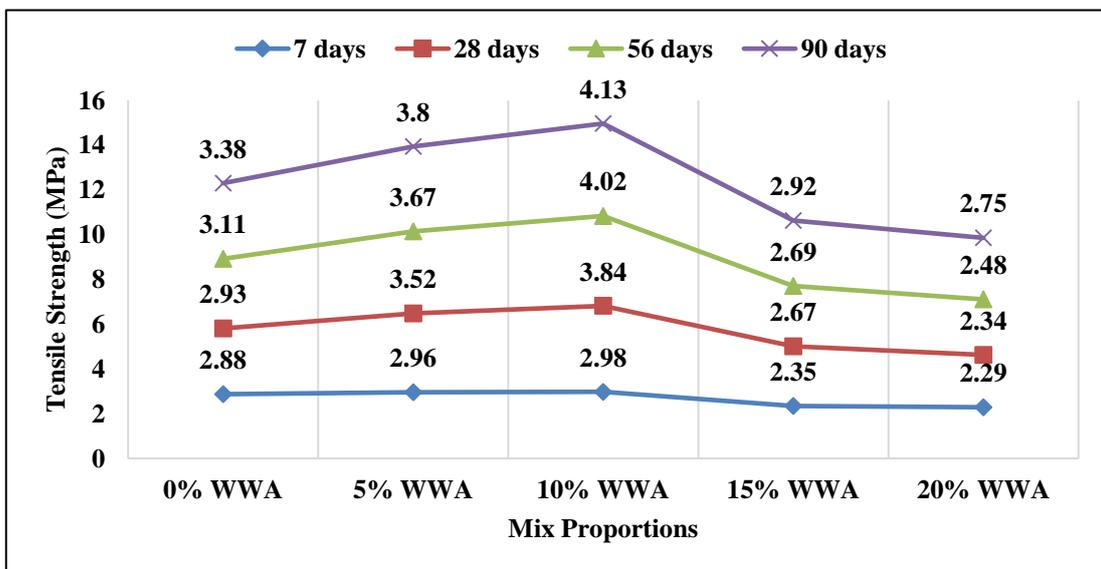
Figure 5- Split Tensile Strength of WWA Concrete
