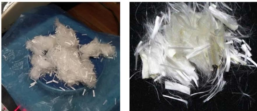
*Fig. 1 – Polyvinyl Alcohol (PVA) Fibres used in the study*
