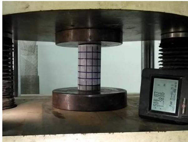
(b) Test setup of compression test
