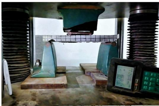
(c) Test setup of flexural strength test
