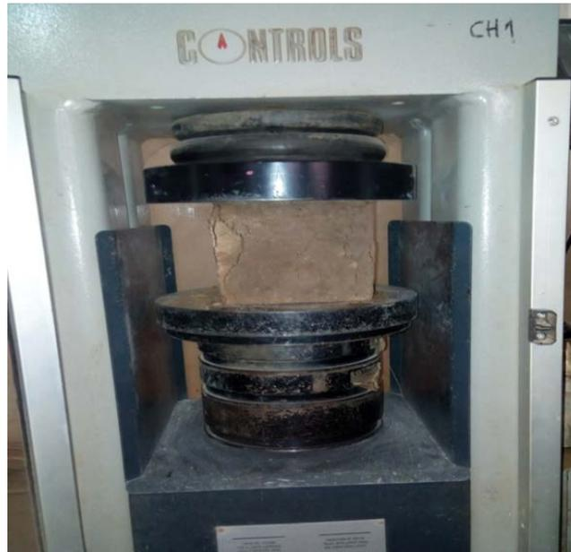
*Fig. 2 - Compressive strength test set-up.*
