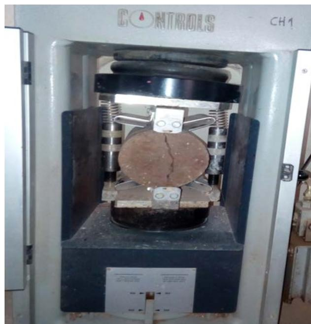
*Fig. 3 - Tensile splitting strength test set-up.*
