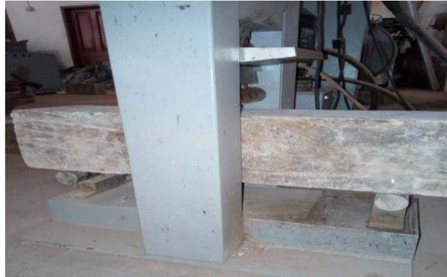
*Fig. 4 - Flexural (3-point load) strength test set-up.*
