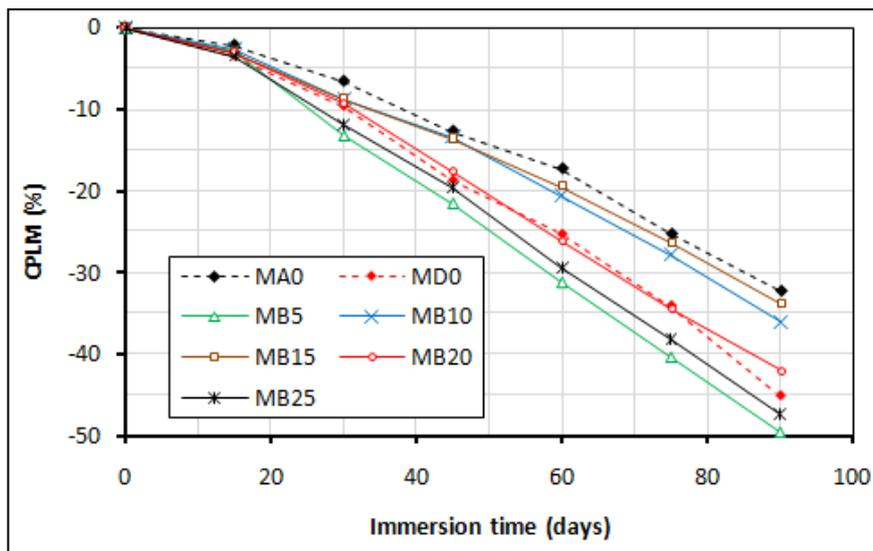
Fig. 9- Mass loss of mortar samples made with CBW due to immersion in sulfuric acid solution
