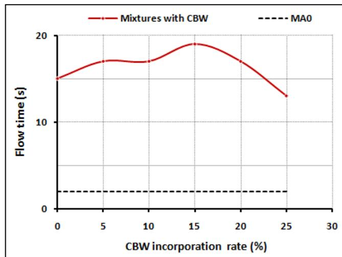
Fig. 3- Variation of workability as a function of the substitution rate
