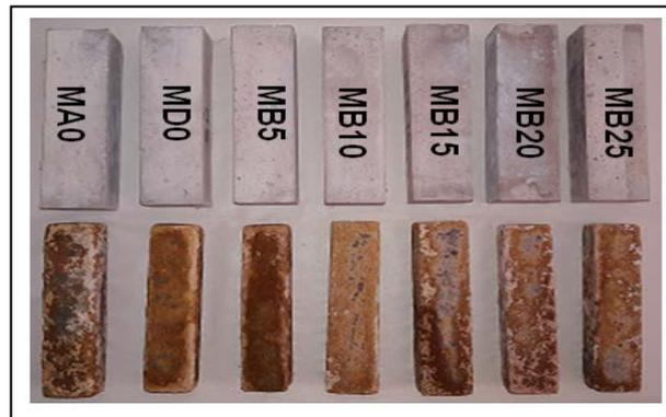
*Fig. 10- Deterioration of CBW samples after 90 days of immersion in 5% H<sub>2</sub>SO<sub>4</sub> solution*
