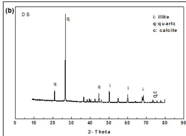
*Fig. 2.b- X-ray diffraction patterns of sand DS*
