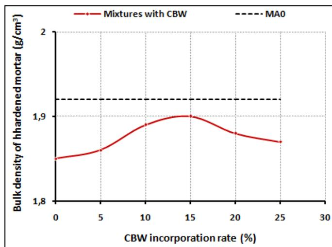
Fig. 5- Effect of CBW incorporation rate on bulk density of hardened mortar
