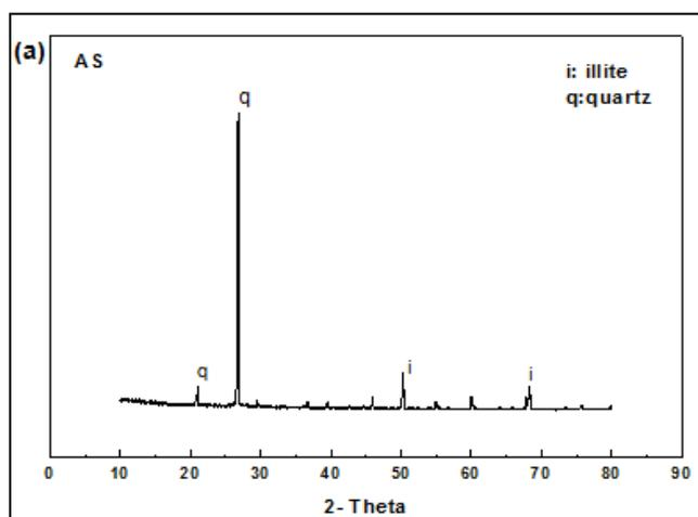
*Fig. 2.a- X-ray diffraction patterns of sand AS*
