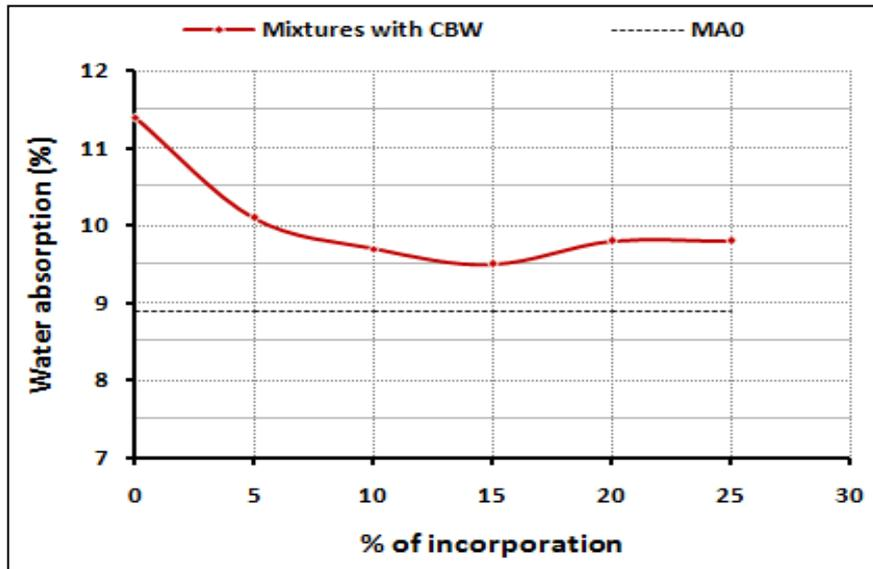
Fig. 8- Effect of CBW amount on water absorption
