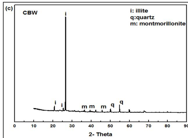
*Fig. 2.c- X-ray diffraction patterns of CBW*
