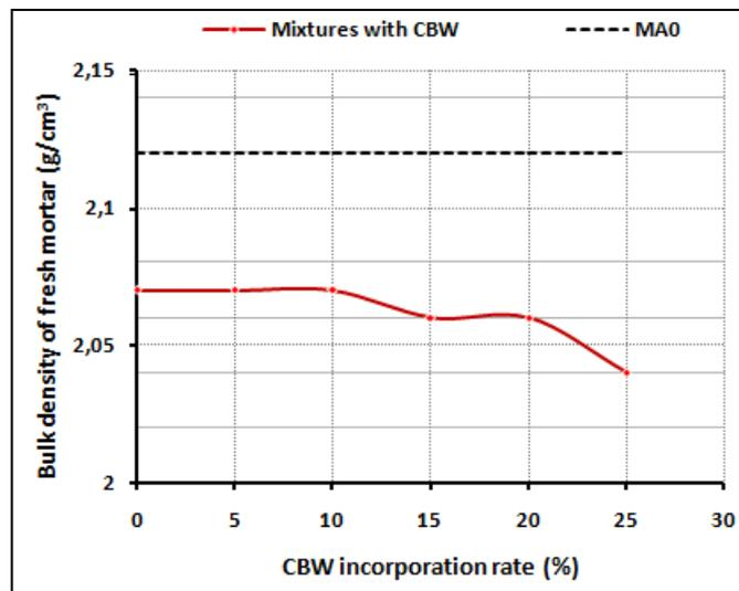
Fig. 4- Effect of the inclusion of the CBW on bulk density of fresh mortar
