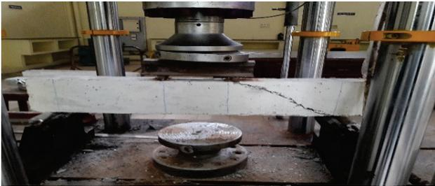
*Figure 22 Failure pattern of RASCC30*
