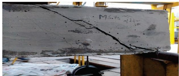
Figure 21 Failure pattern of NASFRSCC70
