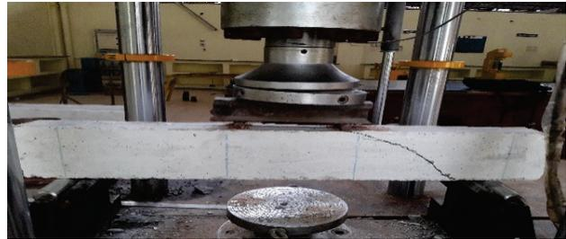
*Figure 23 Failure pattern of RASFRSCC30*
