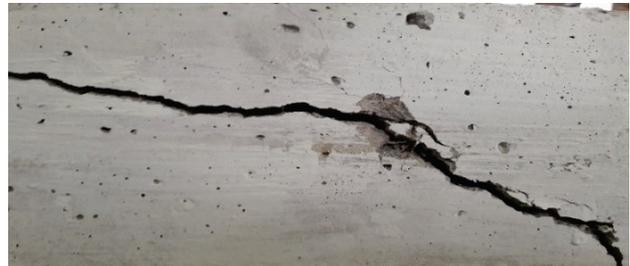
Figure 19 Failure pattern of NASFRSCC30
