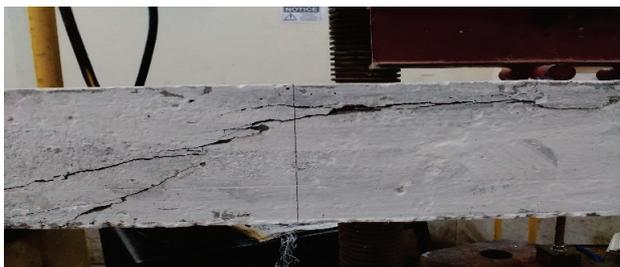
Figure 20 Failure pattern of NASCC70
