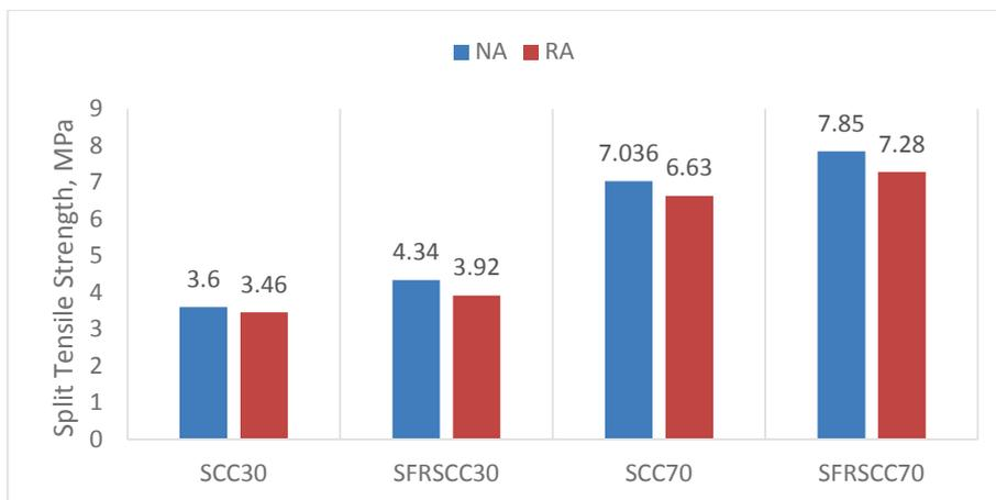
**Figure: 5(b)- Split tensile strength vs Type of concrete (NASCC and RASCC)**
