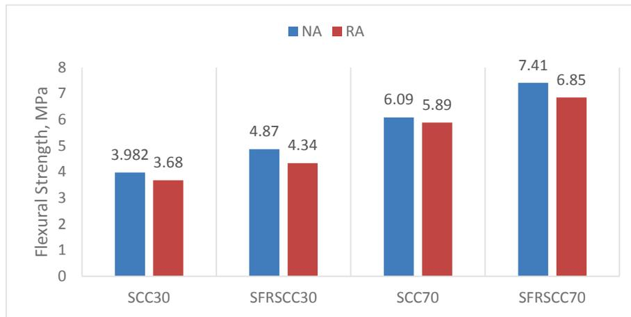
Figure 5(c)- Flexural strength vs Type of concrete (NASCC and RASCC)
