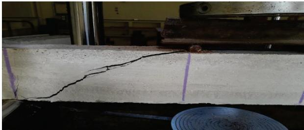
Figure 18 Failure pattern of NASCC30
