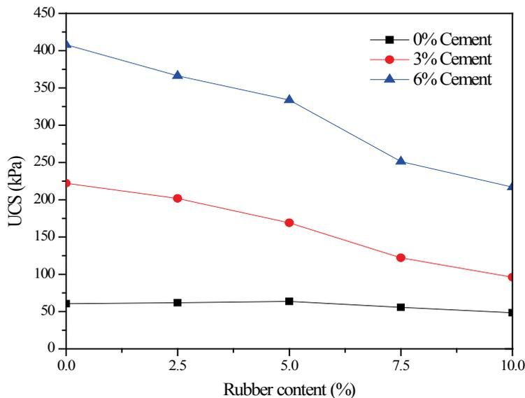
Fig. 5- Effect of cement and rubber content on the UCS of the 28 days cured specimens.
