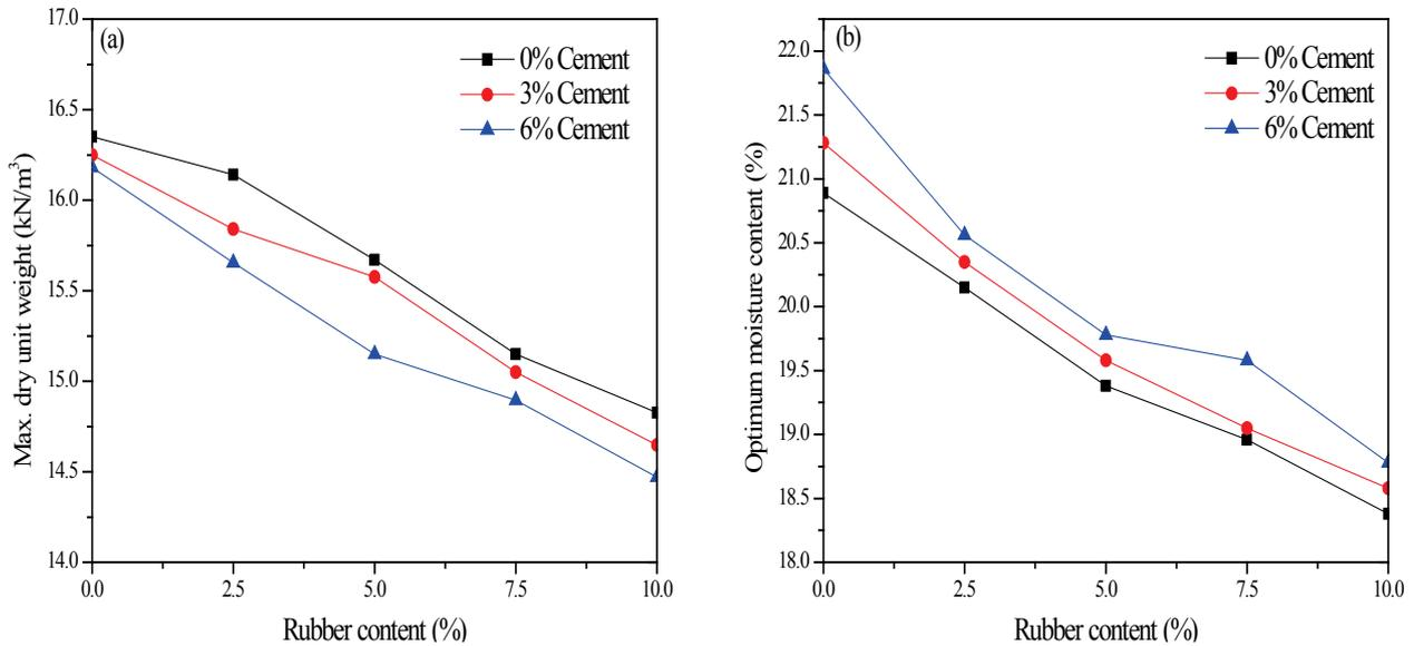
Fig. 4- Effect of cement and rubber content on the (a) maximum dry unit weight; (b) optimum moisture content
