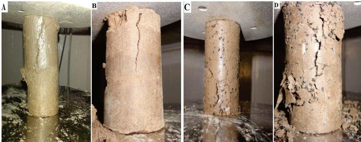
**Fig. 9- Effect of cement and rubber content on the failure characteristics in compression: (a) clayey soil; (b) 6% cement –modified clayey soil; (c) 5% rubber and 3% cement –modified clayey soil; (d) 7.5% rubber and 6% cement- modified clayey soil**
