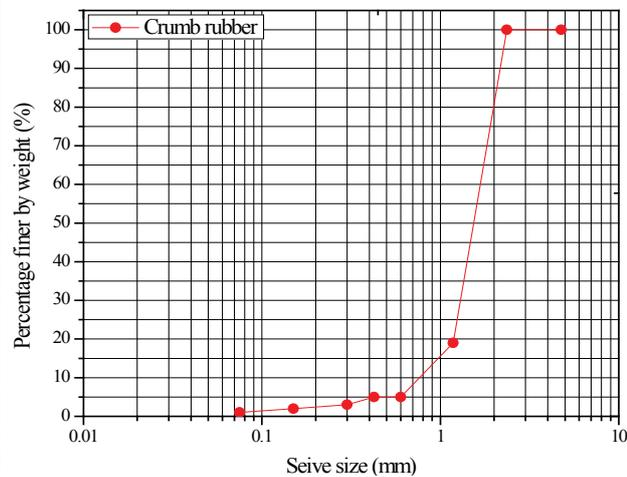
**Fig. 2- Grain size distribution of crumb rubber**
