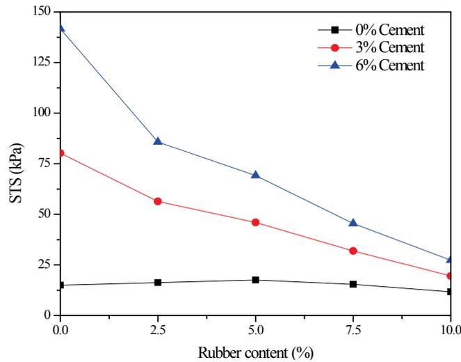
Fig. 6- Effect of rubber content on the STS of the 28 days cured specimens
