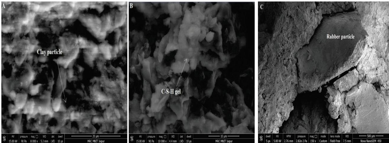
**Fig. 13- SEM images of cement-rubber-modified clayey soil with (a) clayey soil only; (b) 6% cement; (c) 5% rubber and 6% cement.**
