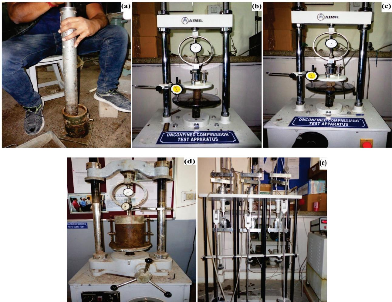
*Fig. 3-Specimen under (a) modified compaction test; (b) unconfined compressive strength test; (c) split tensile strength test; (d) California bearing ratio test; (e) Swelling pressure test*
