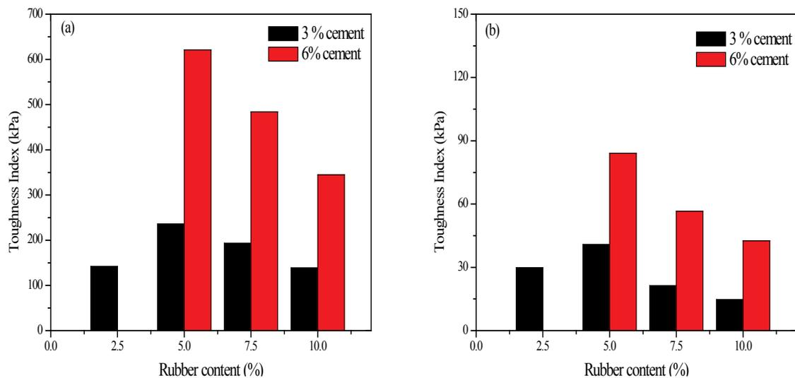
Fig. 8- The effect of cement and rubber content on TI for 28 days cured specimens under (a) UCS; (b) STS test.
