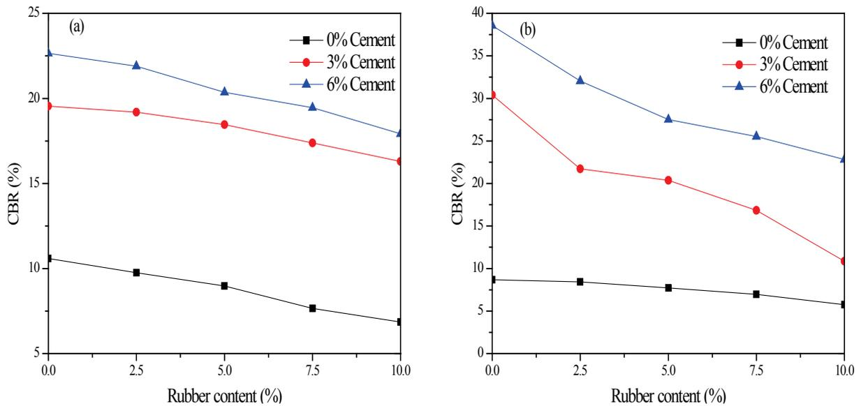
Fig. 11- Effect of rubber content the CBR values (a) Unsoaked condition (b) Soaked conditions
