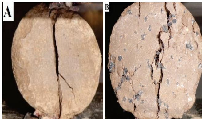
**Fig. 10- Effect of cement and rubber content on the failure characteristics in tension: (a) 6% cement-modified clayey soil; (b) 5% rubber and 3% cement –modified clayey soil.**
