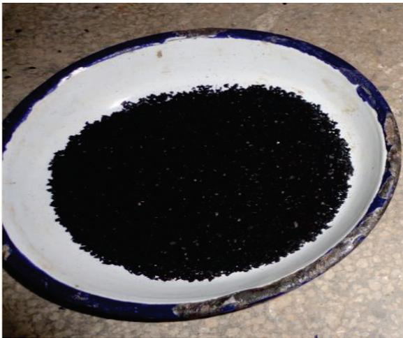
**Fig. 1- Crumb rubber used in the study**
