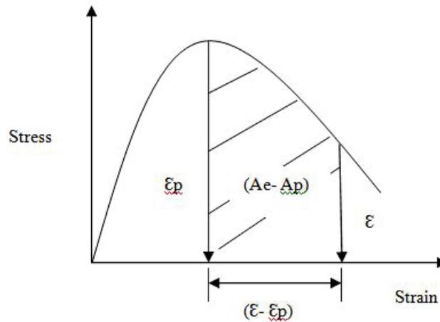
Fig. 7- Typical Stress-strain curves for calculation of TI
