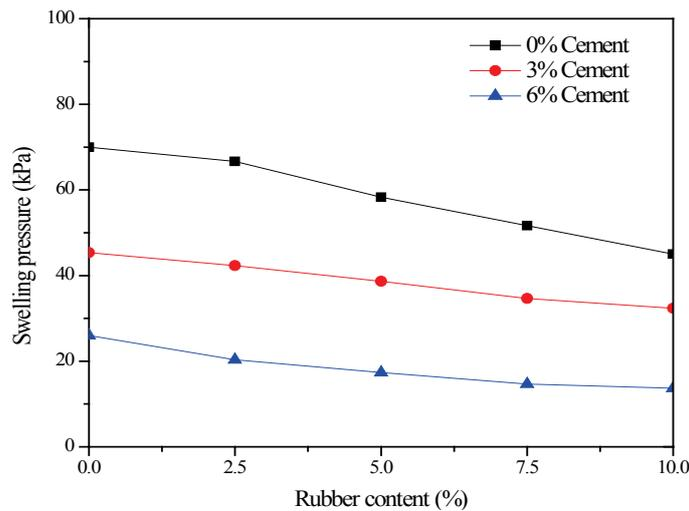
Fig. 12- Effect of rubber content on the swelling pressure
