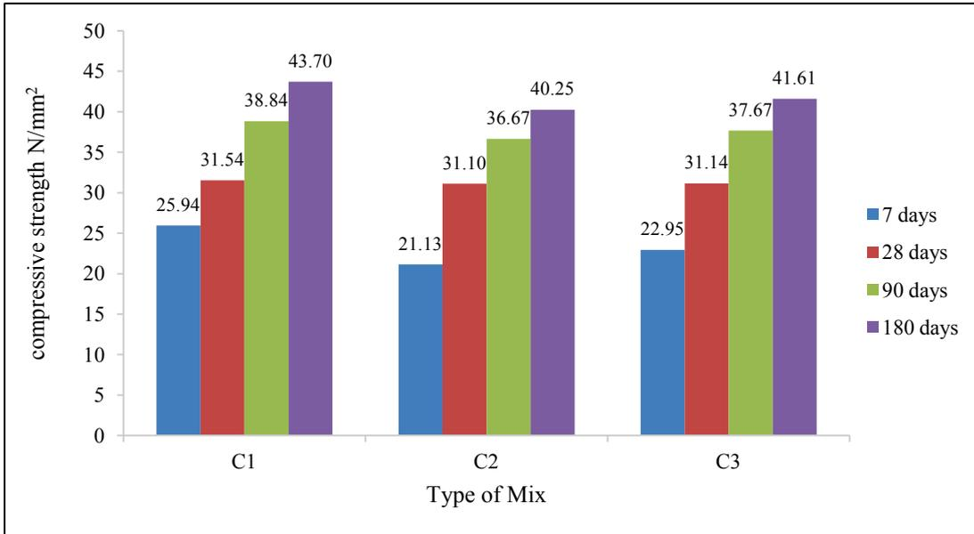
Figure 3 Variation in compressive strength of concrete
