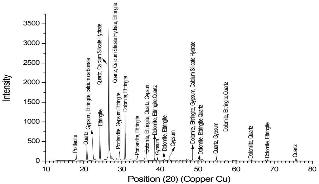
Figure 10 (b) XRD of concrete mix C2 exposed to 5% H<sub>2</sub>SO<sub>4</sub> solution after 90 days
