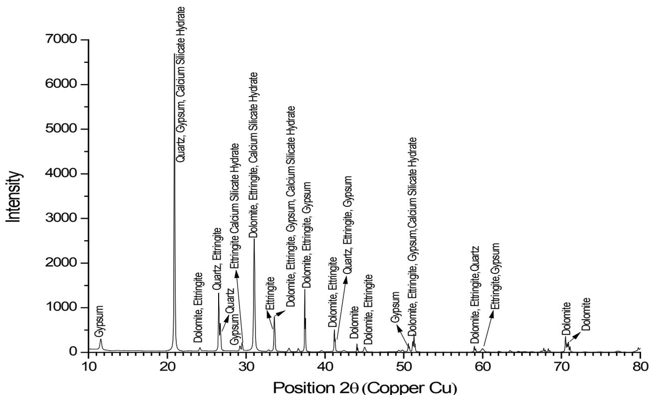
Figure 10 (c) XRD of concrete mix C3 exposed to 5% H<sub>2</sub>SO<sub>4</sub> solution after 90days
