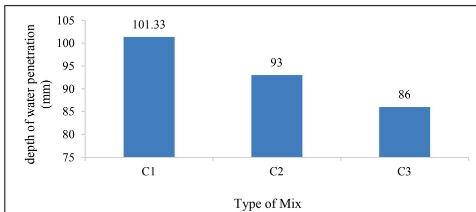
**Figure 2 Variation in depth of penetration of concrete**
