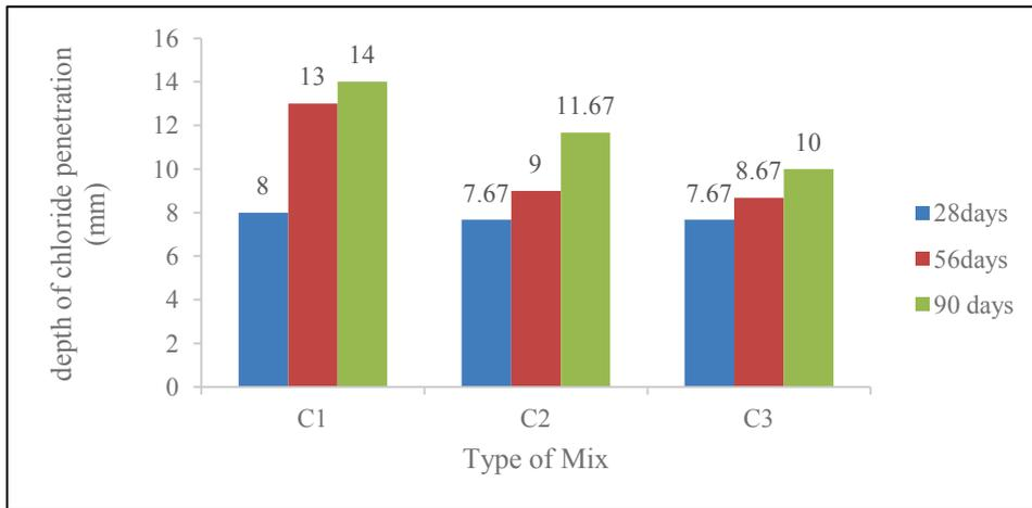
Figure 7 Variation in depth of chloride penetration
