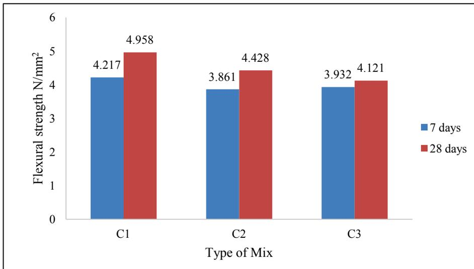
Figure 4 Variation in Flexural strength of concrete
