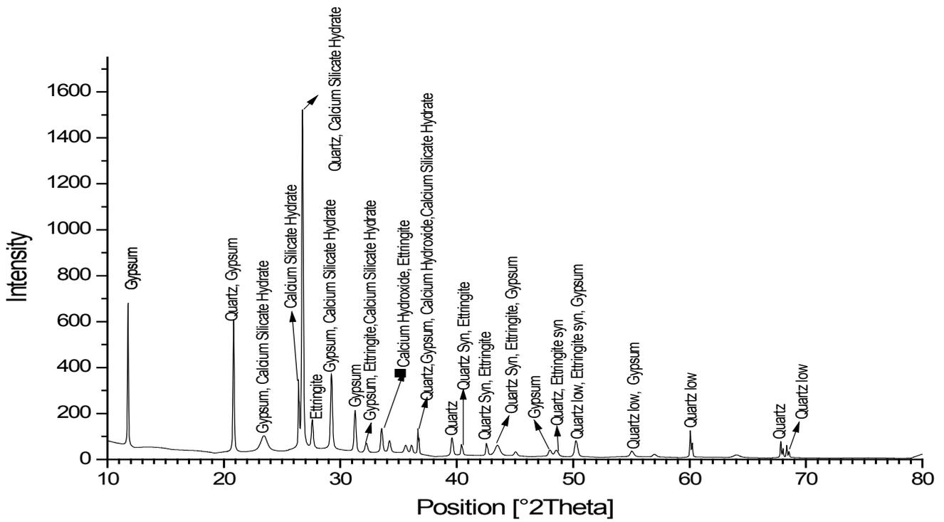
Figure 10 (a) XRD of control concrete exposed to 5% H<sub>2</sub>SO<sub>4</sub> solution after 90 days
