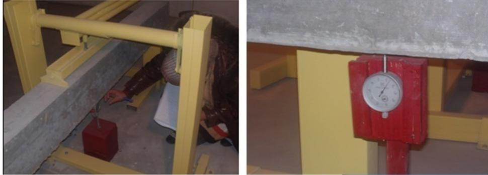
**Fig. 3 – Beam test instrumentation**
