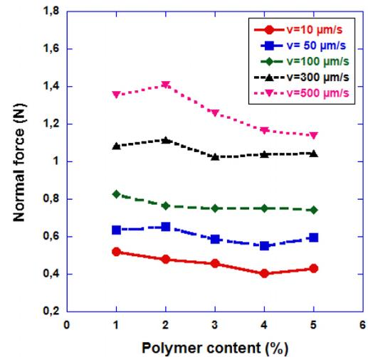
Figure 4: Evolution of the adhesion force versus resin content for different pulling velocities.
