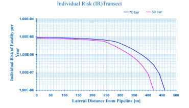
The actual likelihood of a release does not increase at higher pressure, because the pipeline is designed to contain the higher pressures. Fig.5 illustrates the IR transects for the pipeline at the operating pressures.
