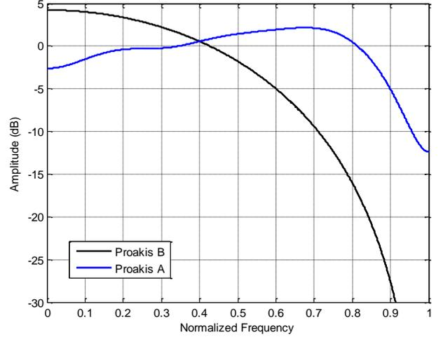
Figure 6. Frequency response of Proakis A and B channels.
