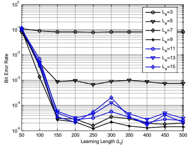
Figure 7. Performance of UTTCM using MMSE equalizer according to the variation of Equalizer response length ( $L_e$ ) and learning sequence length ( $L_l$ ). Parameters of simulation:  $SNR = 26$  dB and 4 decoding iterations.
