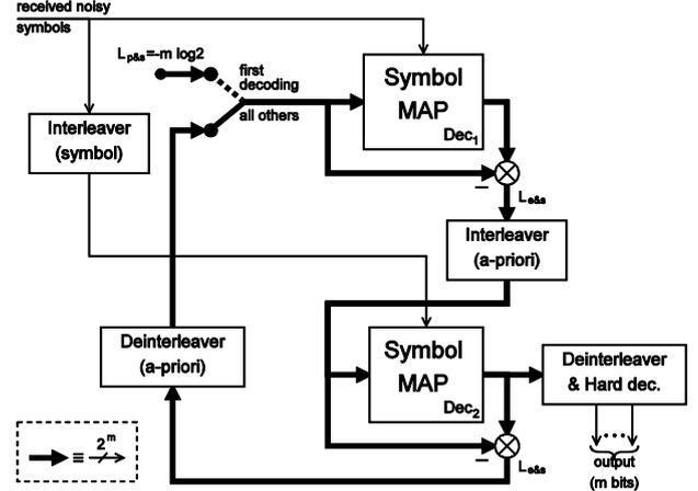
Figure 4. Iterative decoding scheme of UTTCM.
