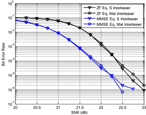
Figure 12. BER Performance of UTTCM over Proakis B channel for 4 decoding iterations using the optimum simulation parameters.
