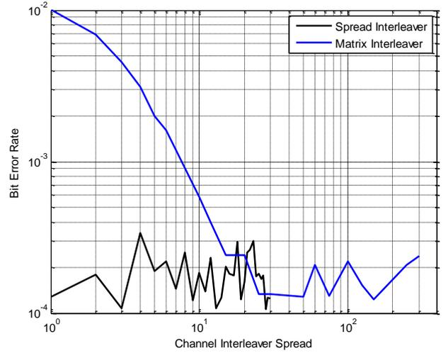
Figure 10. Performance of UTTCM using ZF equalizer according to the variation of channel interleaver spread value ( $S$ ). Parameters of simulation:  $L_e = 7$ ,  $SNR = 23$  dB and 4 decoding iterations.
