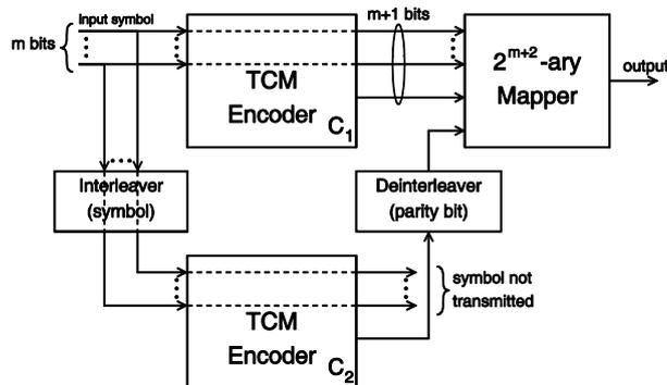
Figure 2. Turbo encoding scheme of UTTCM.
