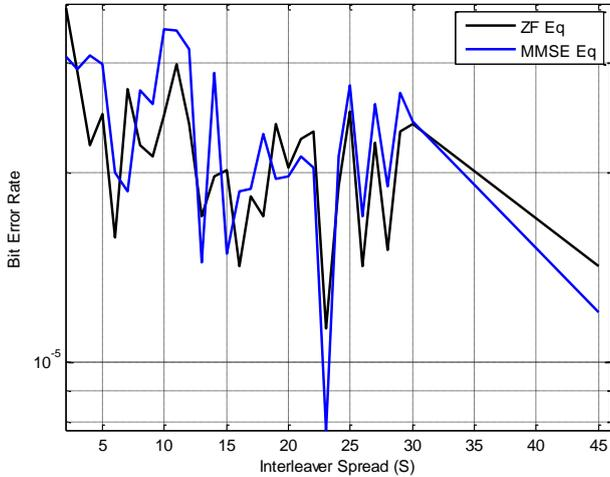
Figure 9. Performance of UTTCM using ZF or MMSE equalizer according to the variation of encoder interleaver spread value ( $S$ ). Parameters of simulation:  $L_e(\text{ZF}) = 7$ ,  $L_e(\text{MMSE}) = 9$ ,  $L_l(\text{MMSE}) = 250$ ,  $SNR = 26$  dB and 4 decoding iterations.
