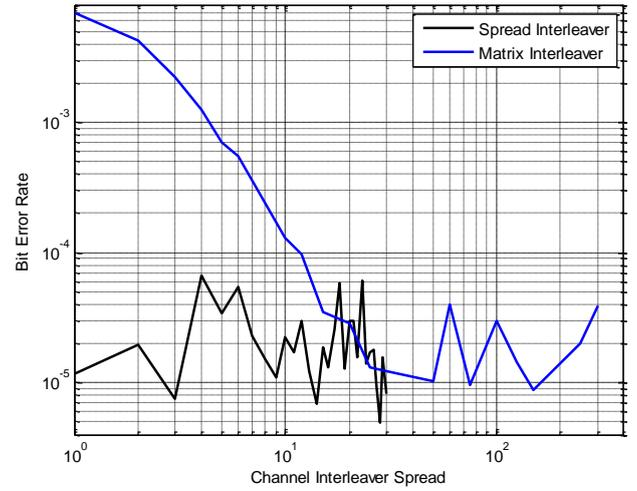
Figure 11. Performance of UTTCM using MMSE equalizer according to the variation of channel interleaver spread value ( $S$ ). Parameters of simulation:  $L_e = 9$ ,  $L_l = 250$ ,  $SNR = 23$  dB and 4 decoding iterations.
