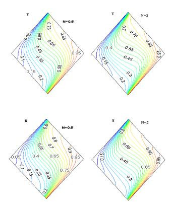
Fig. 3.Isotherms, iso-concentration and streamlines for combined global heat and mass flows, Le = 0.8,  $\alpha$ =  $45^{\circ}$ , Ra = 100, for N =0.5,  $\Psi$ max= 8.9 and N=2,  $\Psi$ max= 14.4.
