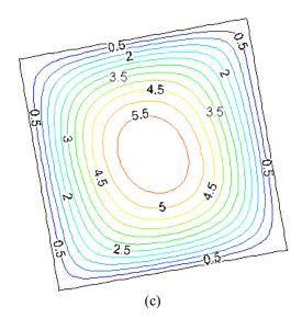
Fig. 2. streamlines for N = 0 (a) Ra=70,  $\alpha$ = 0,  $\Psi$ max= 3.7, (b)  $\alpha$ = 0, Ra = 100,  $\Psi$ max= 2.7, (c)  $\alpha$ =30°, Ra = 100,  $\Psi$ max= 6.
