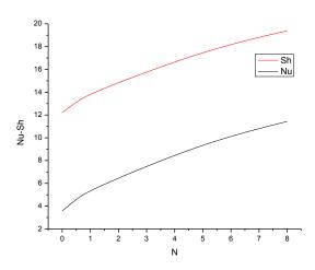
Fig. 4. Global Nusselt and Sherwood numbers as function of the Buoyancy ratio N for  $\alpha=30^\circ$  and Ra=100.
