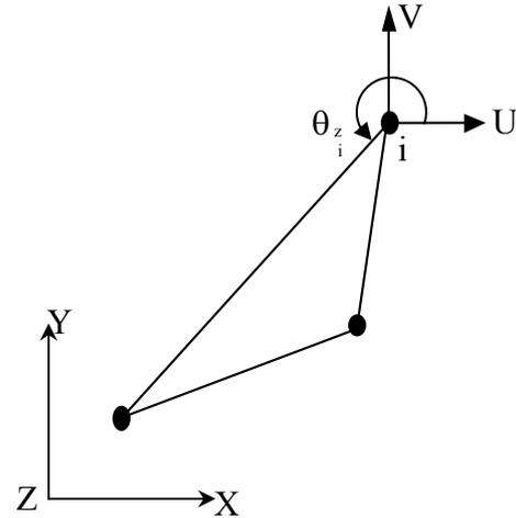
Figure 2 : SBT3 element with drilling rotation
