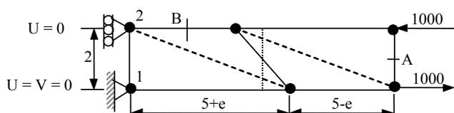
Figure 4c of a cantilever beam; Data and grids. Rotation  $\theta_z$  is free into 1, and 2.
