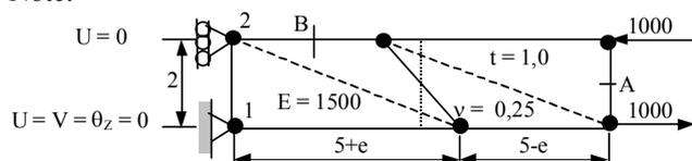
Figure 4a of a cantilever beam; Data and grids. Rotation  $\theta_z$  is free into 2.
