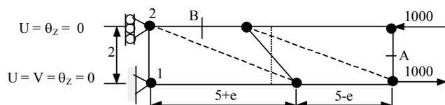
Figure 4b of a cantilever beam; Data and grids. Rotation  $\theta_z$  is fixed into 1 and 2.
