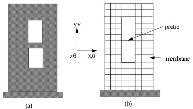
**Figure 1: Structure (shear wall) and its discretization**
