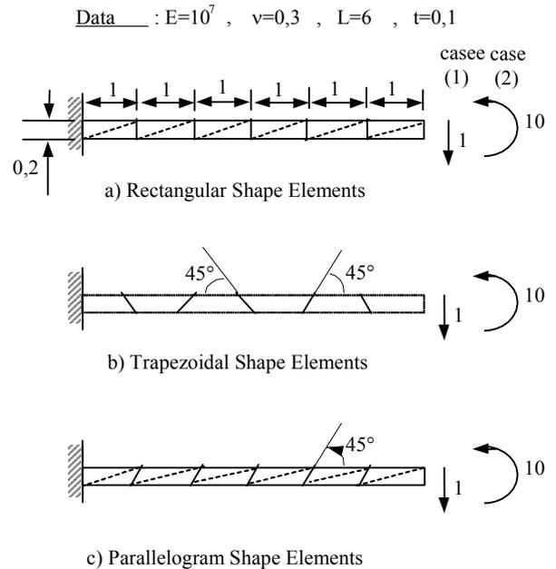
**Figure 5: Slender cantilever beam of MacNeal. Data and grids.**
