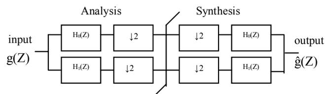
Figure 2 : One-Dimensional DWT
