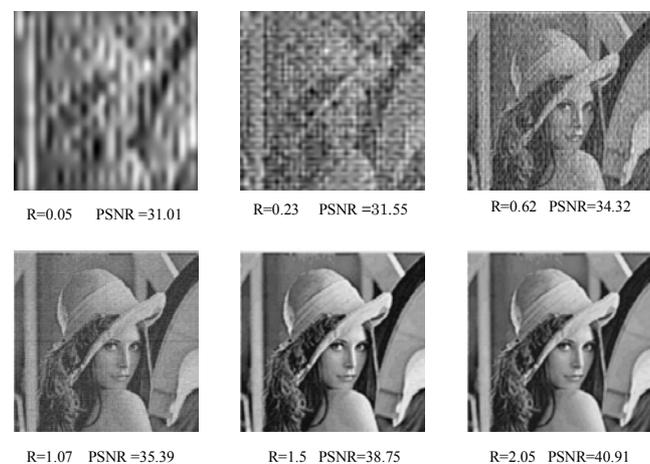
Figure 9 : Effect of bit rate on compression quality
