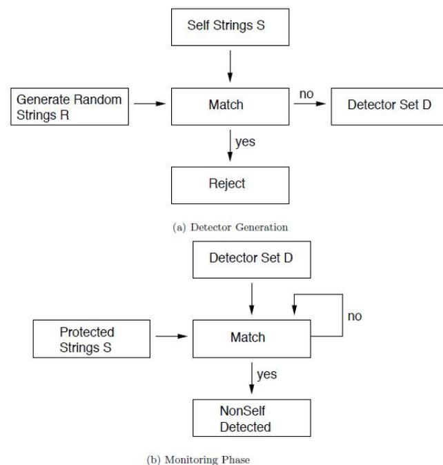
Figure 1: Negative Selection Algorithm by Forrest [7].
