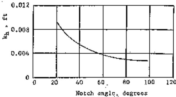
**Figure 1: Depth correction factor  $k_h$  for V-notches of any angle (National Bureau of Standards, Kulin and Compton, 1975).**
