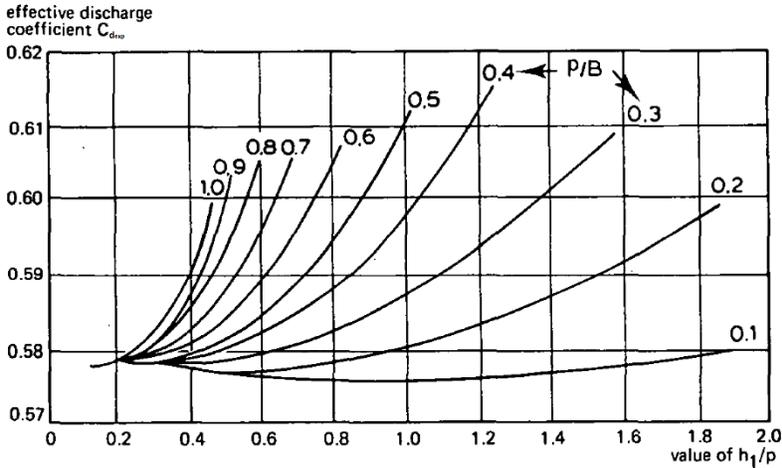
**Figure 3: Experimental discharge coefficient for partially contracted 90-degree V-notches (Kulin and Compton, 1975).**
