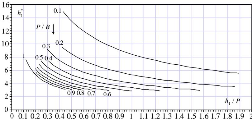
**Figure 4: Variation of  $h_1^*$  with  $h_1 / P$  for some values of  $P/B$  according to Eq. (14b)**
