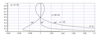
Figure 2: Variation of  $n/n_f$  with h/D in a smooth circular pipe, according to Eq.(30)
