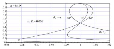
Figure 3: Variation of  $n/n_f$  with h/D in a circular pipe for  $\varepsilon/D=0.001$ , according to Eq.(30)
