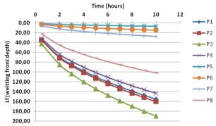
Figure 7: Wetting front depth across the two bank of the river
