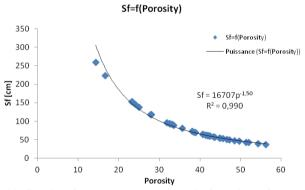
Figure 10: Suction front head expressed in function of the porosity
