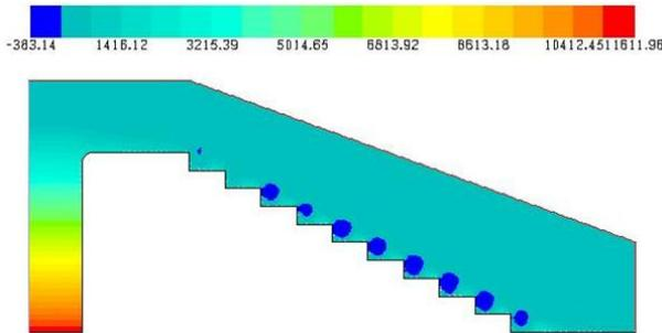
Figure 12 : Contour of static pressure on uniform stepped spillway
