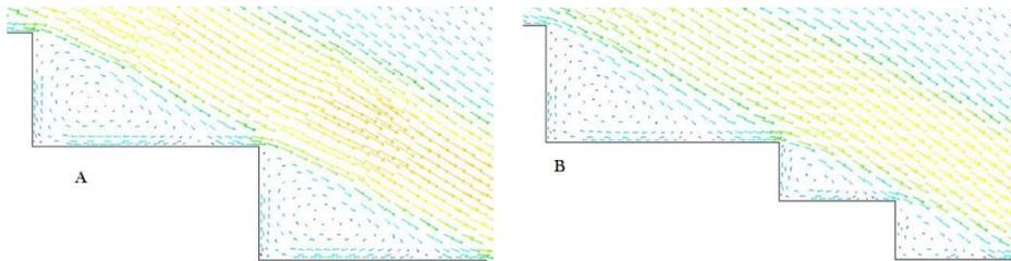
Figure 10 : Recirculation flow in step corner, A: uniform configuration, B: non uniform configuration
