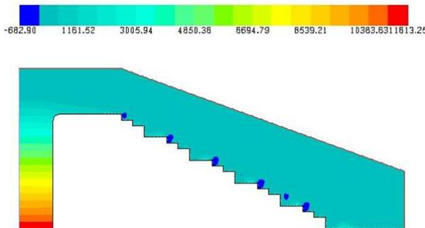
Figure 13 : Contour of static pressure on non uniform stepped spillway
