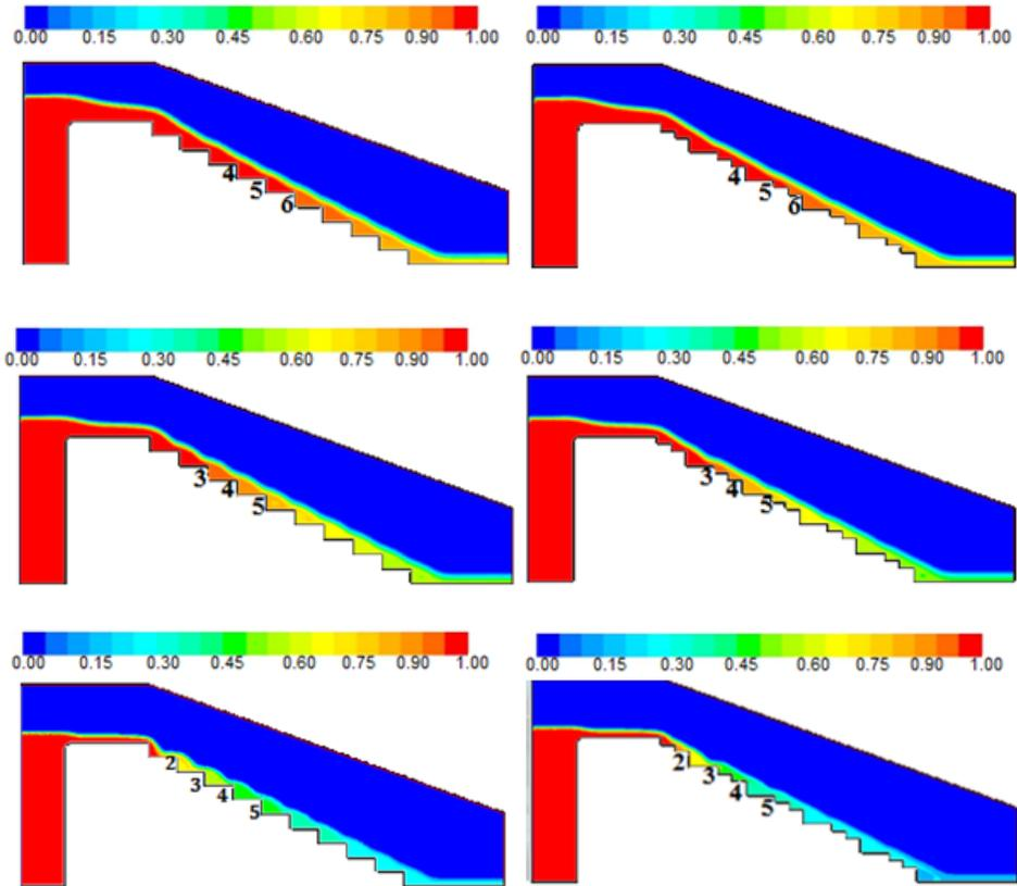
Figure 5 : Numerical void fraction of water on the uniform and non uniform stepped spillways
