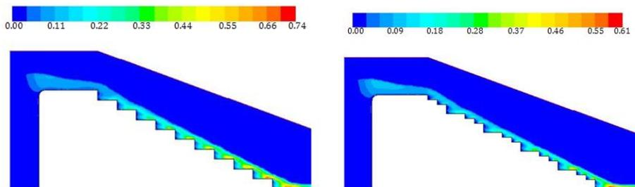
Figure 11 : Turbulence kinetic energy on uniform and non uniform configurations
