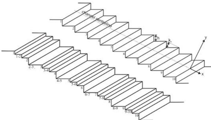
**Figure 2: Uniform and non-uniform stepped spillway configuration**
