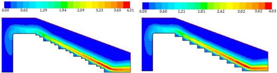
Figure 9 : Velocity distribution on uniform and non uniform configurations
