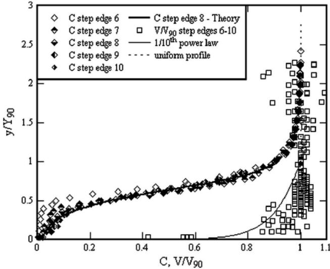
**Figure 8 : Dimensionless velocity and air concentration measured by Felder and Chanson (2011)**
