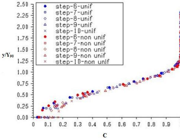
**Figure 6 : Computational air concentration distribution on uniform and non uniform configurations**
