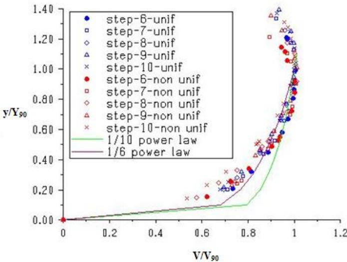
**Figure 7 : Dimensionless velocity on uniform and non uniform configurations**
