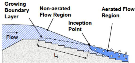
Figure 1: Position of the inception in stepped spillway
