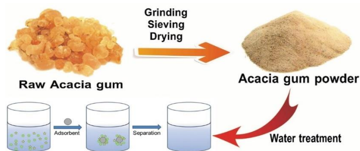
Figure 3. Schema of groundwater treatment by acacia gum.
